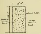
FIG. 22.—HORIZONTAL SECTION OF PIER 10 FT. ABOVE FLOOR OF CRYPT.
